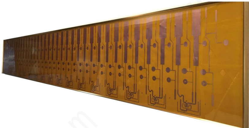
Extra long immersion gold flexible board, finished product size 400mm*2800mm
