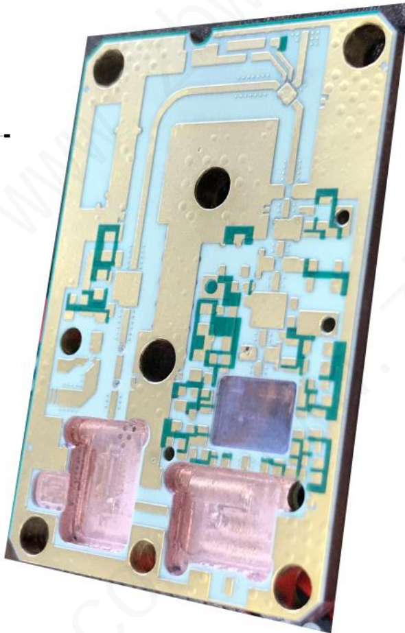
4-layer buried thick copper block HDI various depth step board
